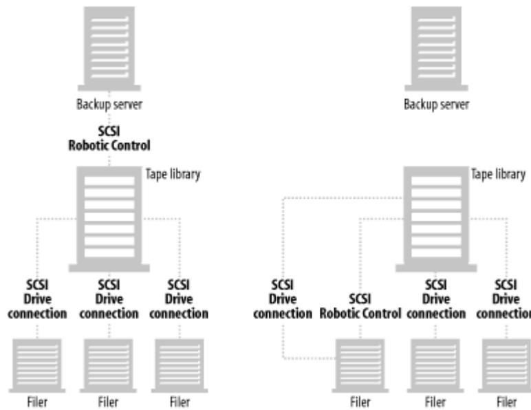
The next level of robotic support allows connecting the tape drives and robotic control directly to the filers, as depicted at the right side of [Figure 7-9](#). This configuration doesn't require the filers or robot to be anywhere near any type of backup server, so it may have advantages in certain environments. It also doesn't require a dedicated SCSI HBA on the backup server, as the configuration at the left side of [Figure 7-9](#) does.
