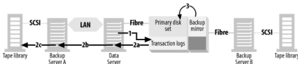
You can also see in [Figure 4-5](#) and [Figure 4-6](#) that the transaction logs don't need to be backed up via the split mirror. The reason for this is that there is no supported methods for backing up transaction logs this way. Therefore, there is no reason to put them on
